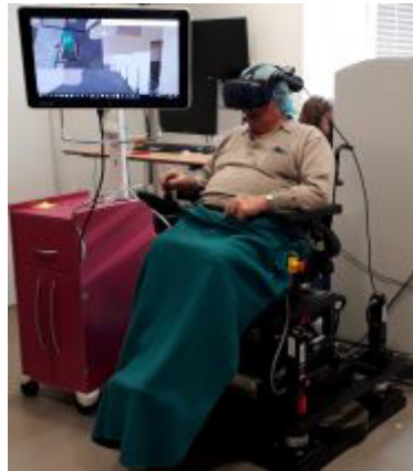
Figure 2. photograph of the power wheelchair simulator with virtual reality helmet
