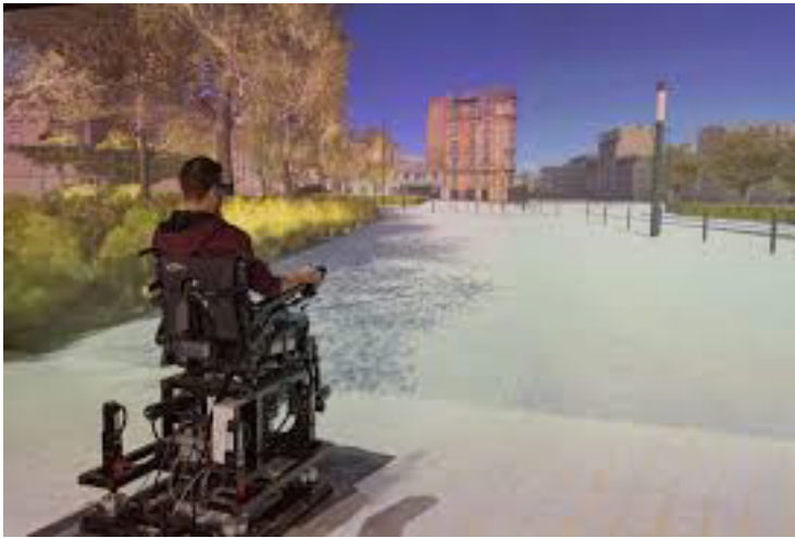
Figure 1. photograph of the power wheelchair simulator in the Immersia platform : view of a street in the Rennes center
