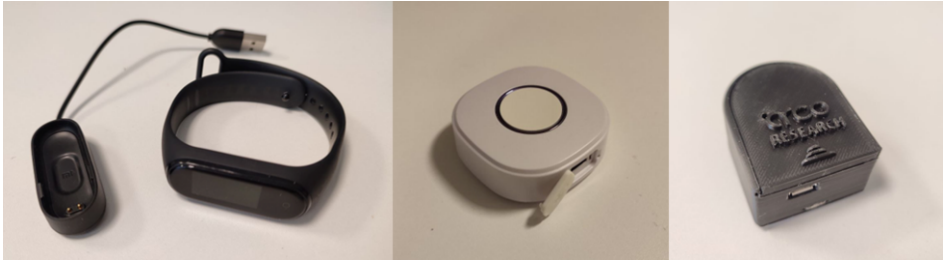
Figure 2. Wearable devices of the use case under study: activity smart band (left), emergency button (center) and fall detector (right)
