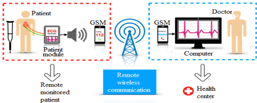
Figure 1. The audio-conversion and transmission of the sonified ECG signal.
