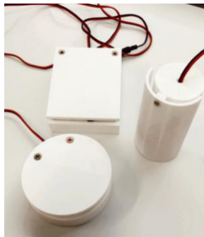
Figure 1. Low-Cost Switches created by workgroup 1
