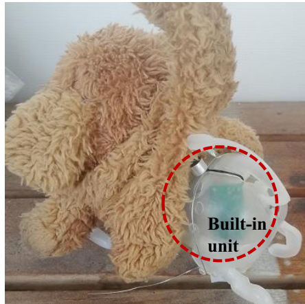
Figure 5. Favorite toys remodeling with sound switch.
