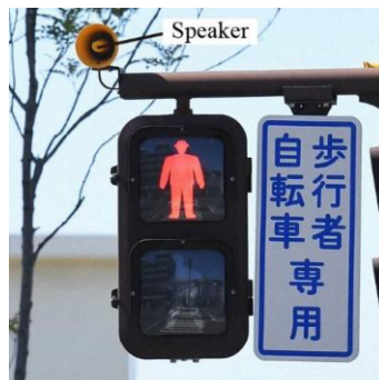
Figure 2. Traffic lights with sound guidance
