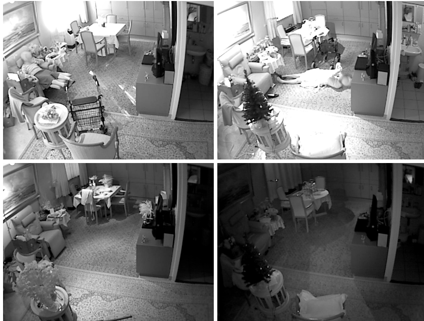
Fig. 2. Examples of video frames with different illumination. Upper left: Sunlight causes overexposure at window. Upper right: Localized overexposure caused by halogen lamps. Lower left: Same room with minor overexposure. Lower right: Frame recorded at night using near infrared.
