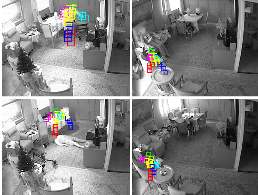
Fig. 5. Examples of the output of a state-of-the-art person detector [28]. Upper left panel: Successful detection of human pose. Upper right and lower panels: Failed to detect pose of the person. (Green : head, yellow : torso, violet : left arm, light blue : right arm, red : left leg, dark blue : right leg)
